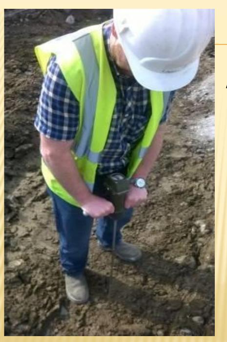
Assessment of Ground Conditions at **Base Level** Penetrometer cone test
